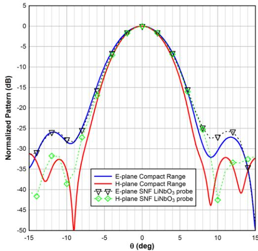
Figure 7. Detail of the main beam and first sidelobes for the measured patterns.
