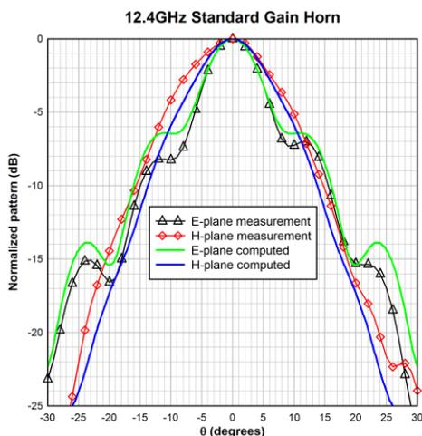
Figure 3. Comparison of measured and computed data for a SGH at 12.4 GHz.
