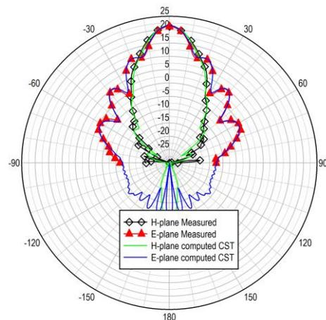
Figure 1. Pattern for the two principal planes at 8.2 GHz. The measured data is transformed from -90° to 90°
