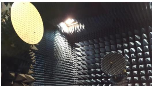
Figure 4. The flat, slotted array antenna mounted to the AUT positioner in the SNF range. Notice the two slots covered with copper tape.
