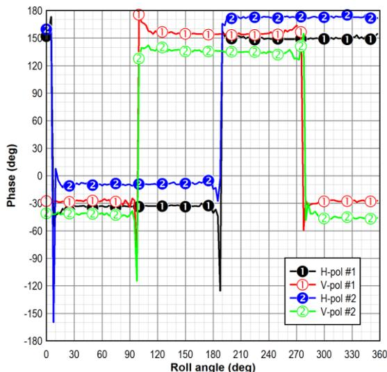
Figure 5. Phase response of polar near-field cuts for two different acquisitions and two different polarizations.
