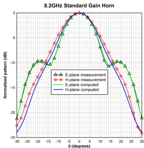
Figure 2. Comparison of measured and computed data for a standard gain horn at 8.2 GHz.
