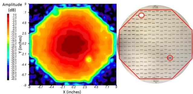
Figure 8. Field at the aperture. The antenna is shown in the figure. Notice the location of the taped slots and the disturbances of the aperture fields caused by these taped slots (dimensions are in inches).
