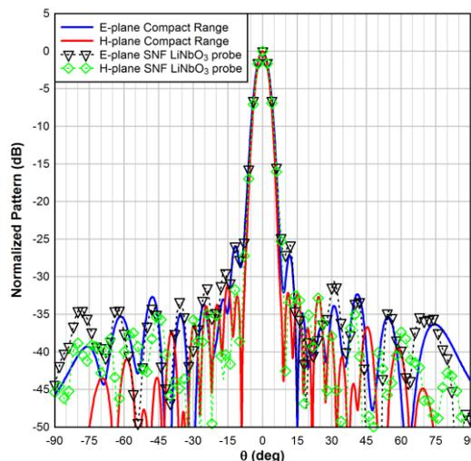
Figure 6. Comparison of the far field data obtained from the near-field data measured using the photonic probe and the compact range data reported in [7].
