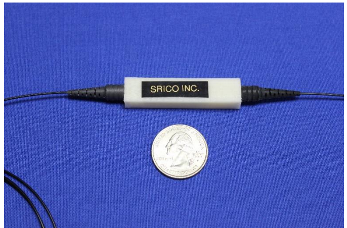
Figure 1. A Lithium Niobate MZI inside its package compared to a 25-cent US coin.
